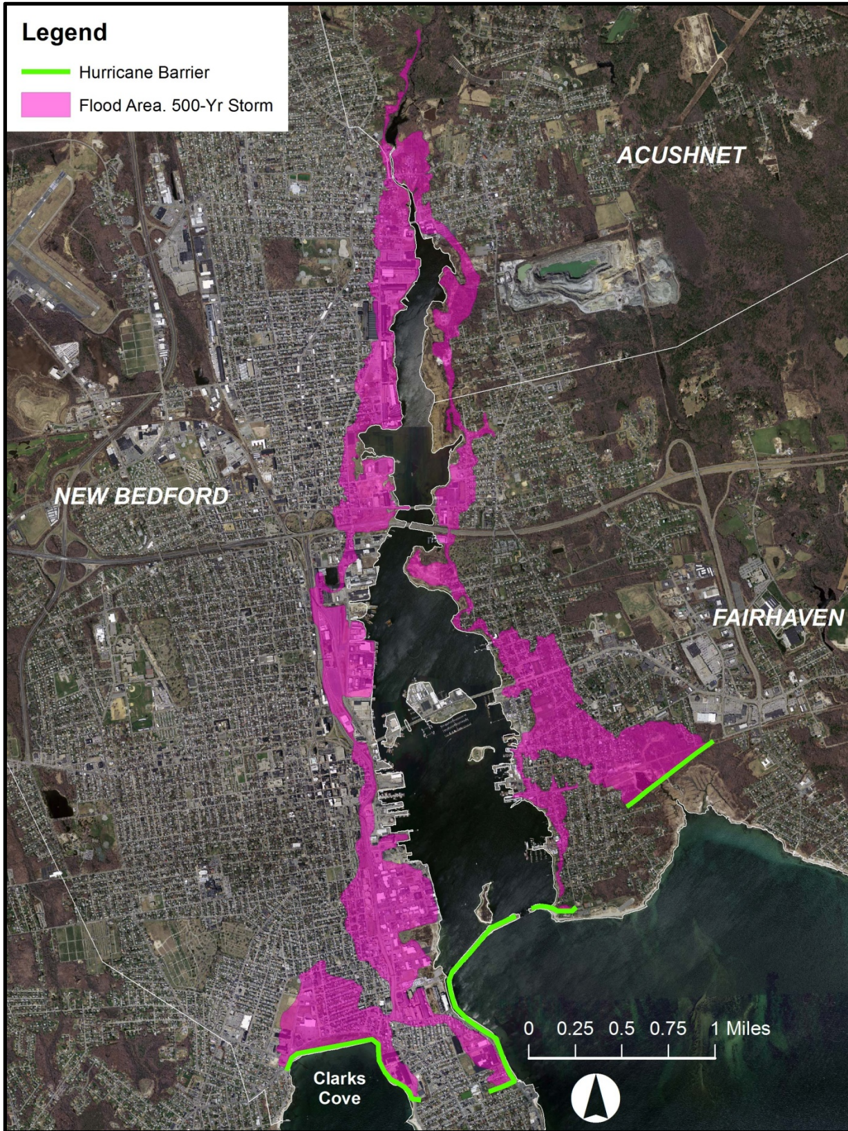
Fig. 4. New Bedford – Fairhaven Hurricane Barrier and 500-yr Floodplain. The New Bedford-Fairhaven Hurricane Barrier (green lines). The areas shaded magenta are in the 500-yr floodplain of the 2009 FIRMS and represent additional flooded areas caused by the overtopping of the barrier, and flooding behind it to roughly a 14-ft elevation.
