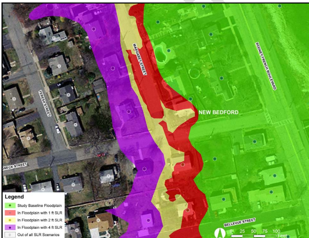
Fig. 3. Structure Assignment in Floodplain Expansion Areas with Different Sea Level Rise Scenarios. Multiple structures (outlined in yellow), if present on a parcel, were converted to label points representing the position of the largest structure. If no structure was present on the GIS coverage, a label point was created for the parcel. The position of these points were used to initially place the primary structure in a flood zone scenario. If a house was crossed by several scenarios, the point location was adjusted to place the building in the lowest elevation zone.
