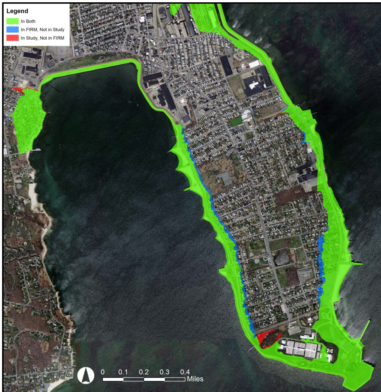
Fig. 5. Comparison of FIRM 100-yr Floodplain to Adjusted Baseline Floodplain in the south end of New Bedford. Figure shows the adjusted baseline floodplain conditions adopted in this study, and how it differed from the 2009 FIRMs 100-year (1% annual risk) coastal floodplain. Area inside the Hurricane barrier had negligible differences between the two coverages. Inland floodplain areas were excluded from the analysis.
