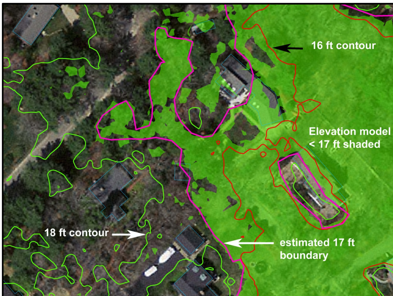
Fig. 2. Mapping Base Flood Elevations BFEs with odd numbered values. In areas where the base flood elevation was set to an odd number value and elevation contours wide spaced, the TIN raster digital elevation model files were coded to match the same base flood elevation boundaries. In this image, a floodplain scenario (shaded green, right) was used to estimate a 17-ft contour (shaded magenta).
