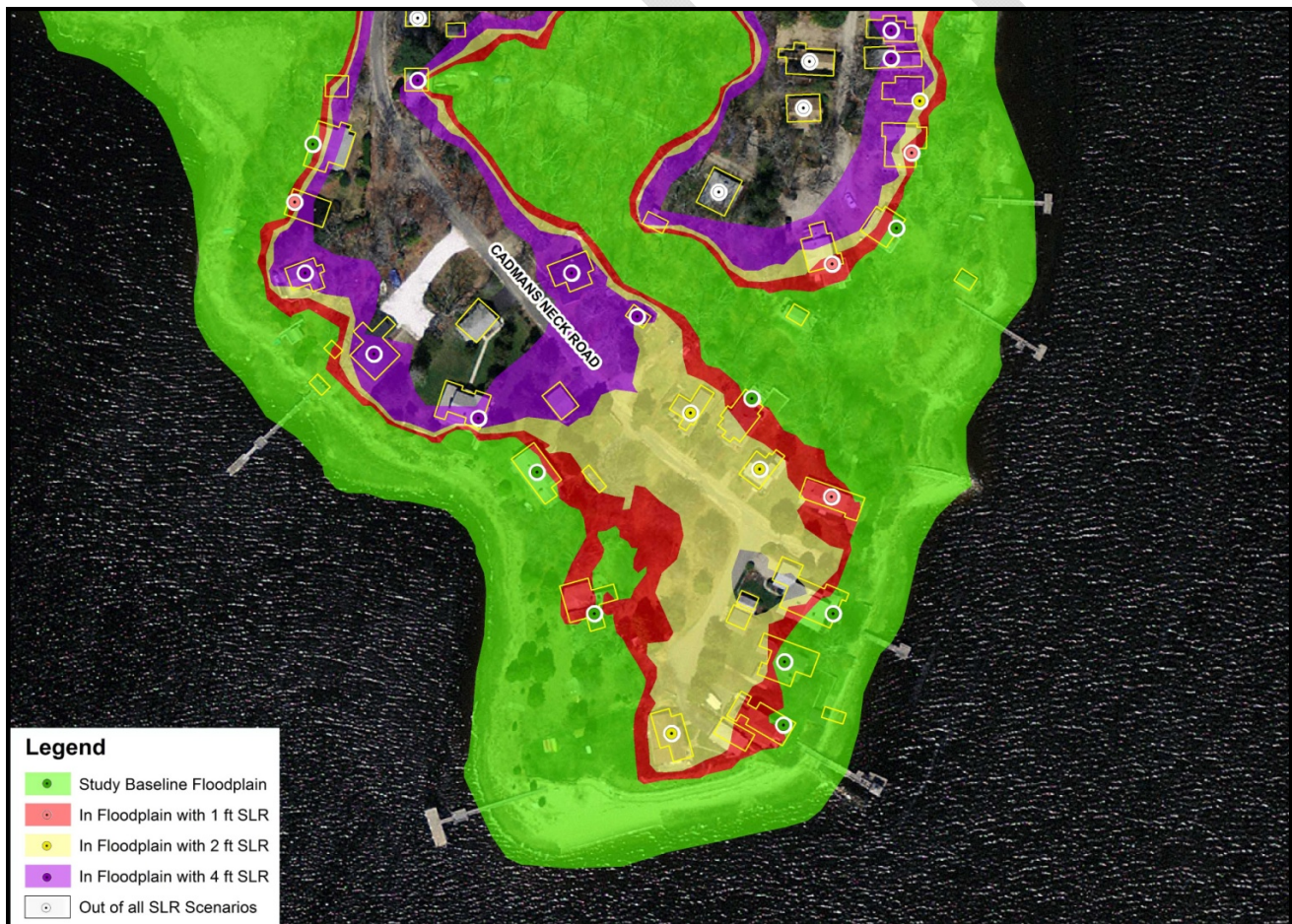
Fig. 3. Structure Assignment in Floodplain Expansion Areas with Different Sea Level Rise Scenarios. Multiple structures (outlined in yellow), if present on a parcel, were converted to label points representing the position of the largest structure. If no structure was present on the GIS coverage, a label point was created for the parcel. The position of these points were used to initially place the primary structure in a flood zone scenario. If several scenarios crossed the footprint of a house, the point location was adjusted to place the building in the lowest elevation zone.
