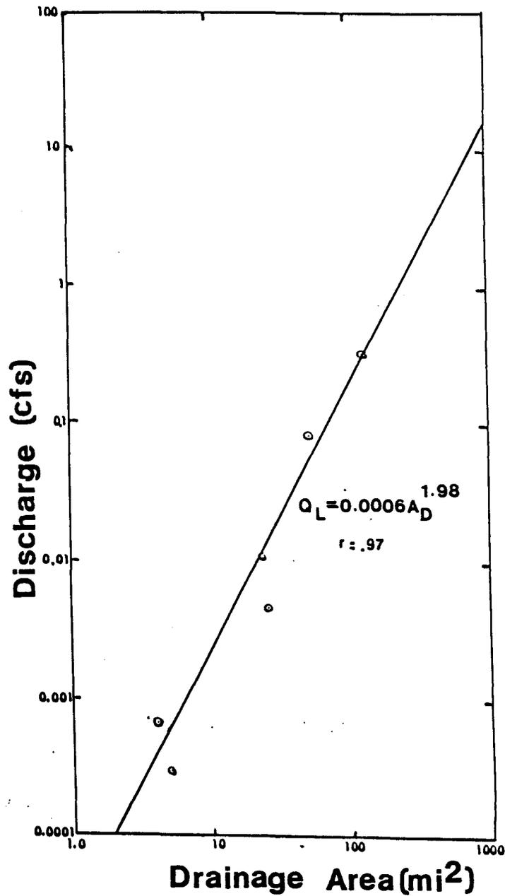
Figure 20. Ten-year low flow analysis of rivers in southeastern Massachusetts and northeastern Rhode Island, from long-term USGS stream discharge data. The line indicates the lowest stream discharge that will occur in a ten year recurrence interval, for any size drainage area in the region. The equation is derived from a regression analysis of the low flow data.
