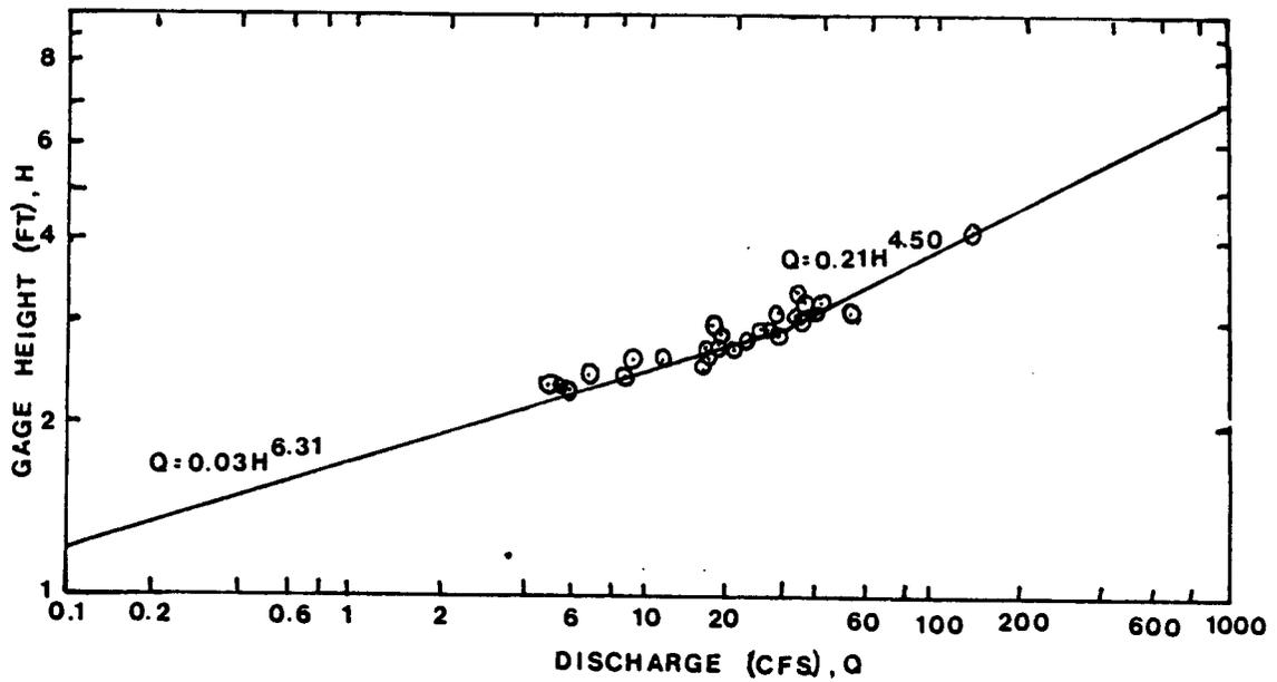
Figure 6. Rating curve for the East Branch stream gage, derived from measurements of stream discharge and stage. The lower portion of the curve represents stream stage at less than bankfull stage and the upper portion of the curve stream stage at greater than bankfull stage. Once the relationships have been established, stream discharge for any gage height may be estimated from the curve or from the regression equations (Kelly et al., 1986).
