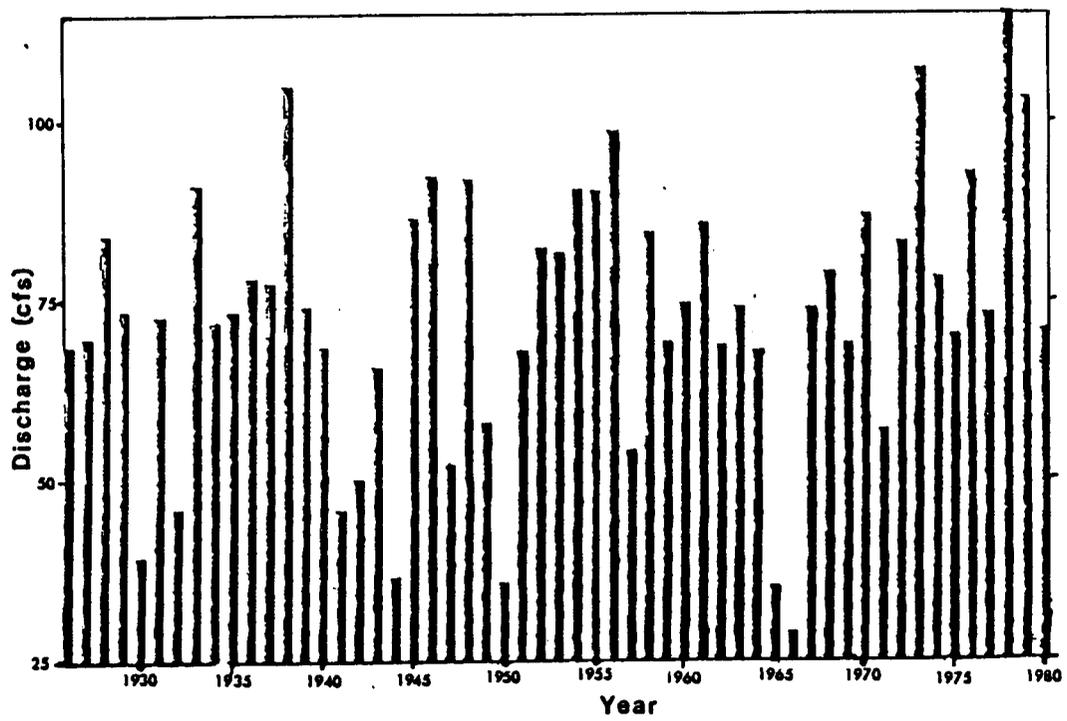
Figure 14. Histogram of annual discharges for the Wading River at Norton, MA for the period 1926 to 1980.
