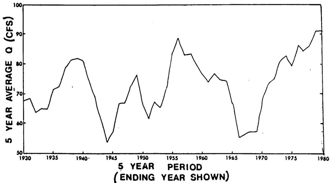
Figure 15. Plot of 5-year running average of annual discharges for the Wading River at Norton, MA, for the period 1930 to 1980. The plot indicates the average of the annual discharges for consecutive 5 year periods, revealing longer term climatic patterns. The curve indicates that the period after 1965 was a particularly dry period.
