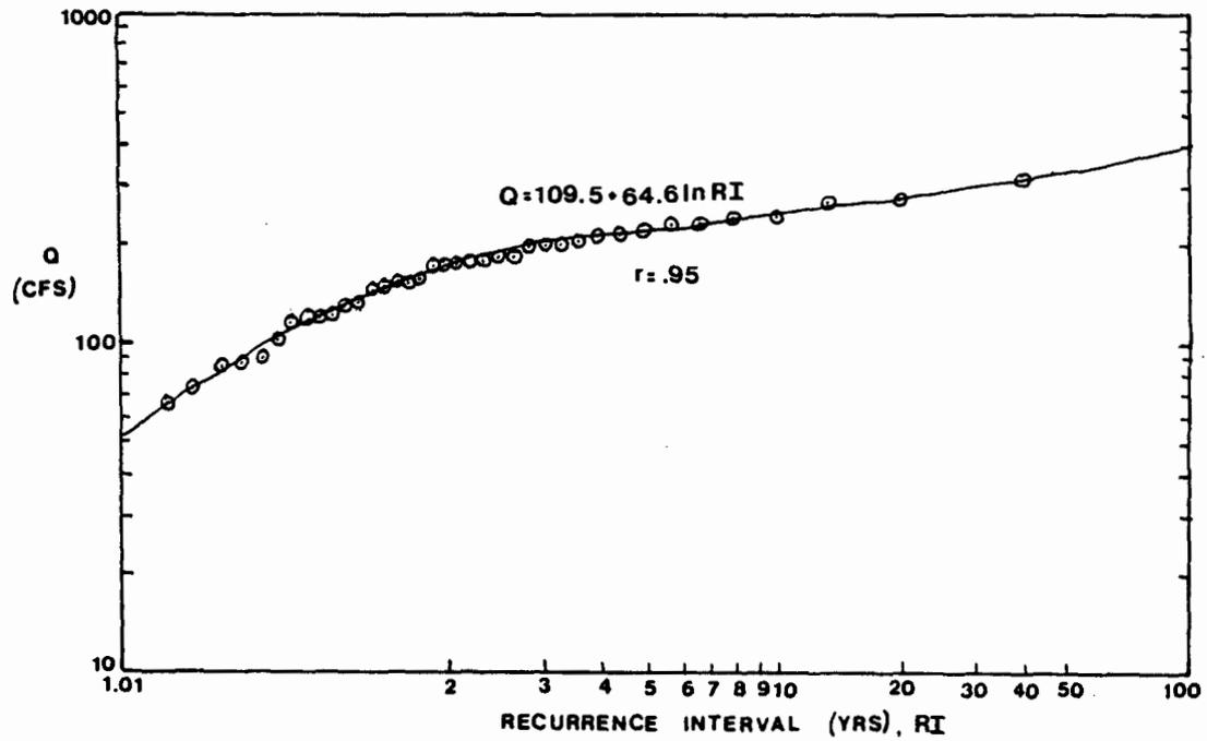
Figure 16. Flood frequency curve for Adamsville Brook, RI, for 1941-1978. The discharge of the annual floods during this period are plotted versus recurrence interval. The discharge of a flood of any recurrence interval may be estimated from the curve or from the regression equation.
