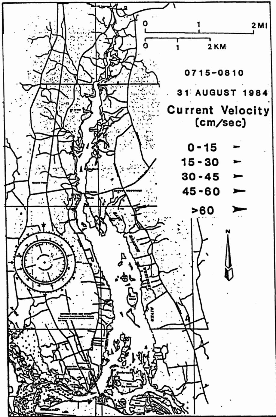
Figure 26. Current velocity magnitudes and directions for eight stations in the East Branch during the period 0715 to 0810 on August 31, 1984, indicated by the arrows shown in the channel. The lack of a uniform direction for the currents indicates the contorted circulation pattern throughout the East Branch.
