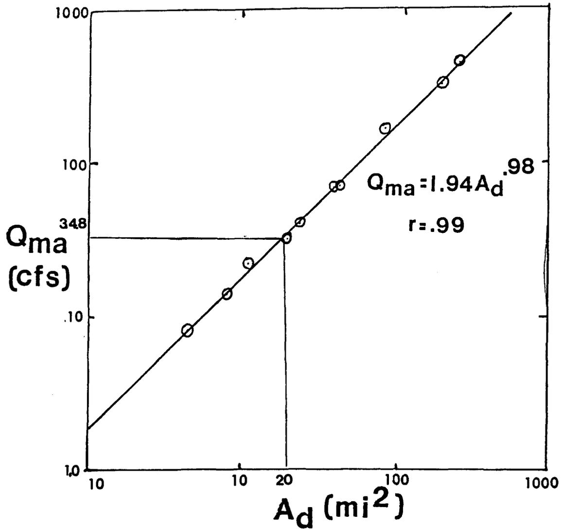
Figure 7. Drainage area-mean annual discharge relationship for southeastern Massachusetts and northeastern Rhode Island, derived from long-term USGS records of mean annual discharge for ten stream gages. The mean annual discharge for any size drainage area in the region may be estimated from the curve, for example, a drainage area of 20 square miles will have a mean annual discharge of 34.8 cfs.
