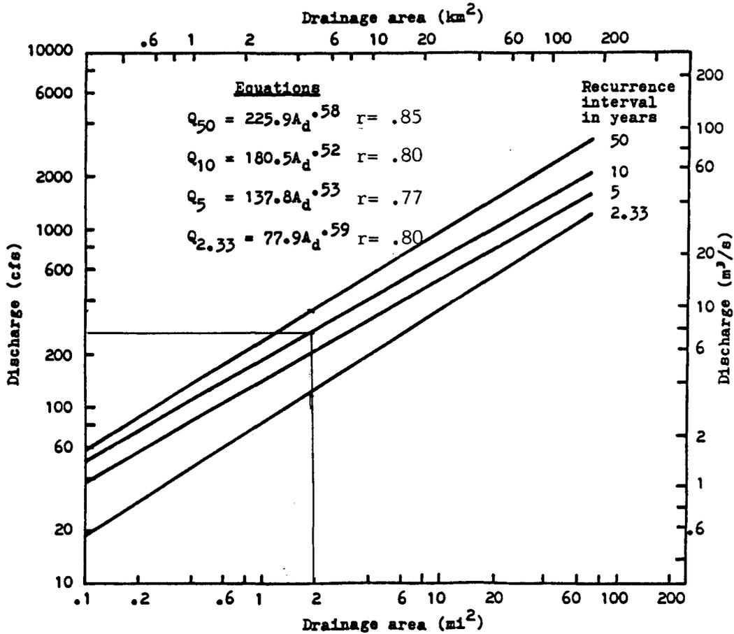
Figure 18. Drainage area and flood discharge relationships for rivers in southeastern Massachusetts and northeastern Rhode Island, from long-term USGS stream gage data. The example indicates that a 10 year recurrence interval flood in a drainage basin of 2 square miles will have a discharge of approximately 260 cfs.
