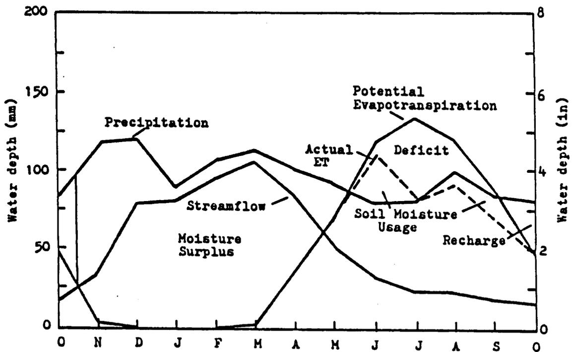
Figure 8. Long-term water budget for the region of the East Branch, derived from precipitation and temperature data from Fall River, MA, and stream discharge information from Adamsville, RI, showing the long-term average changes in precipitation, streamflow, evapotranspiration, and soil moisture (Kelly et al., 1986).
