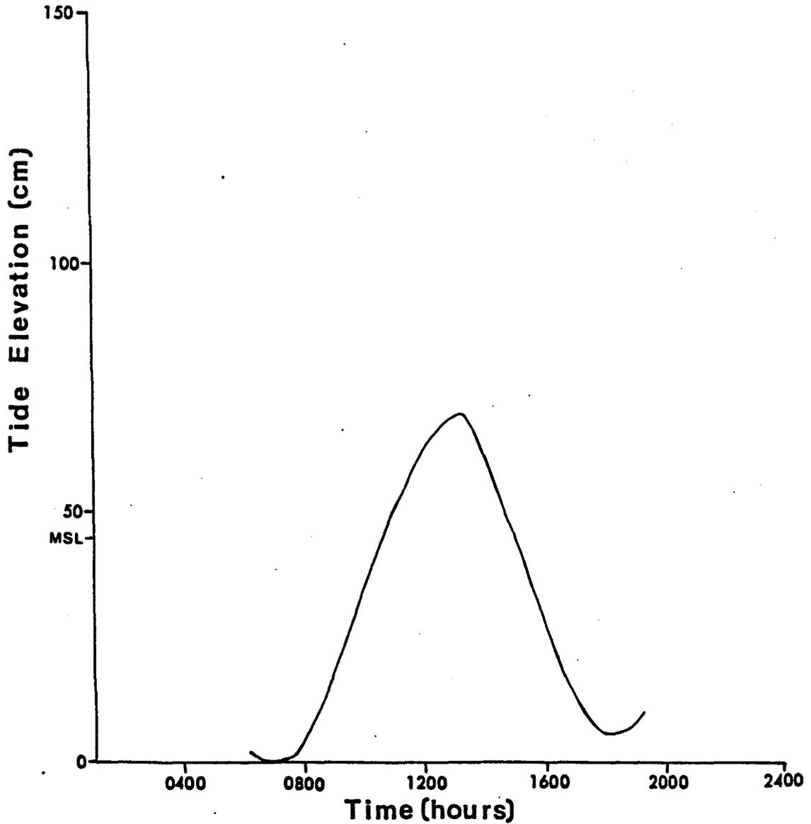
Figure 23. Tide curve for Westport Point on May 25, 1985. The curve indicates the relative rise and fall of the tide during the time period indicated and the total range of the tide for this date (68 cm). Mean sea level for Westport Point relative to this tide occurred at 46 cm above the lowest tide.
