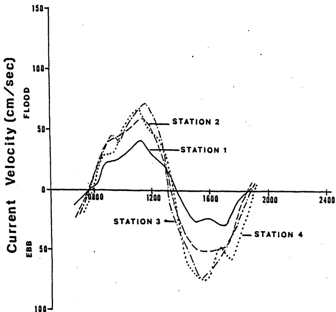
Figure 24. Current velocity curves for four stations at Westport Point on May 25, 1985. The curves indicate the current velocity during the ebb and flood tides for each of the stations. Stations 3 and 4 had the greatest velocities.
