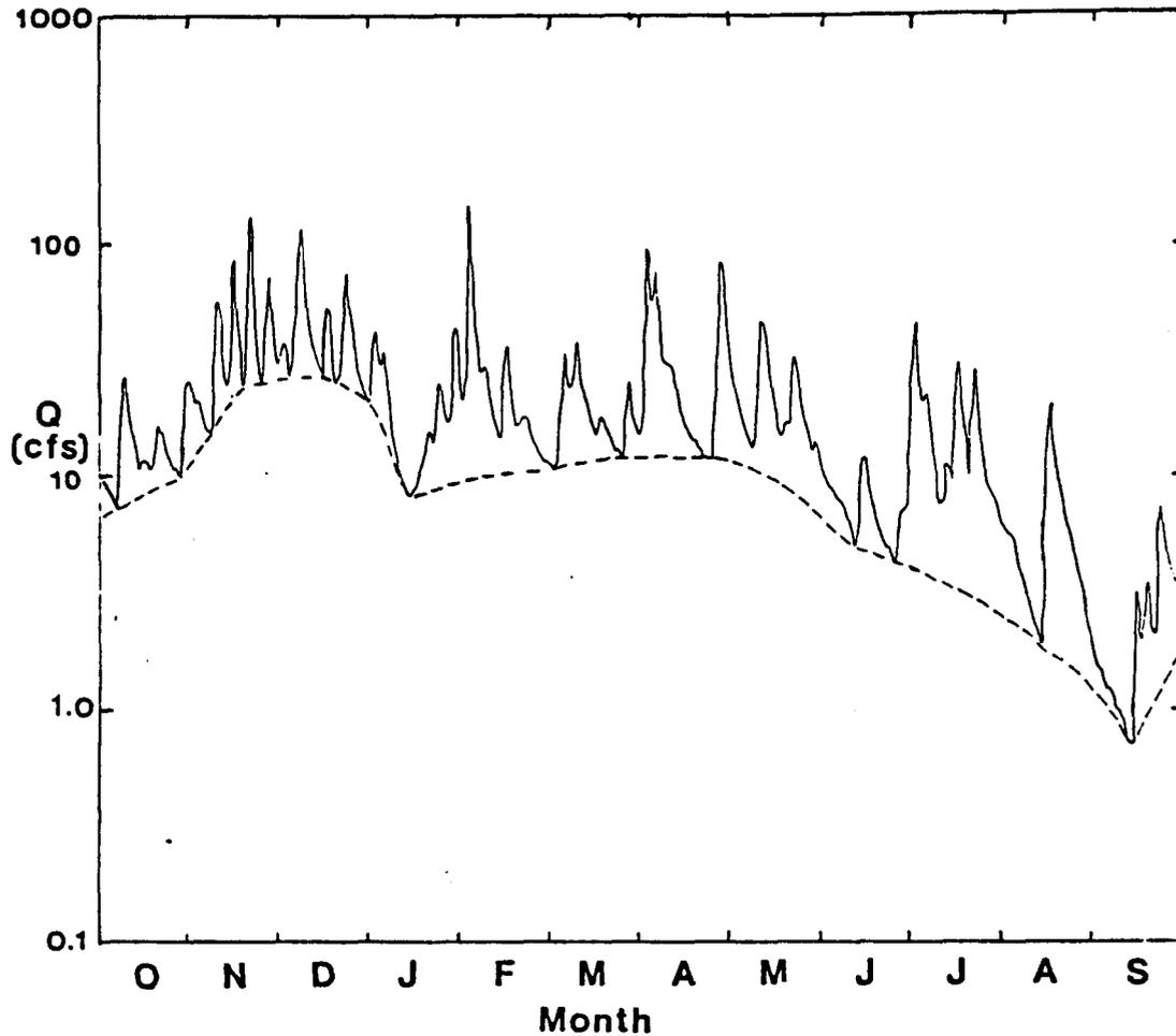
Figure 11. Annual hydrograph for Adamsville Brook, RI, for Water Year 1973, showing the yearly fluctuation in stream discharge (solid line) and in groundwater baseflow (dotted line). This Water Year was a particularly wet year.
