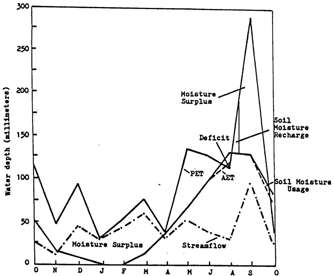
Figure 9. Water budget for 1985 for the East Branch, derived from precipitation and temperature data from several towns in the region, and stream discharge information from Adamsville, RI, showing the actual fluctuations in precipitation, streamflow, evapotranspiration, and soil moisture (Kelly et al., 1986).
