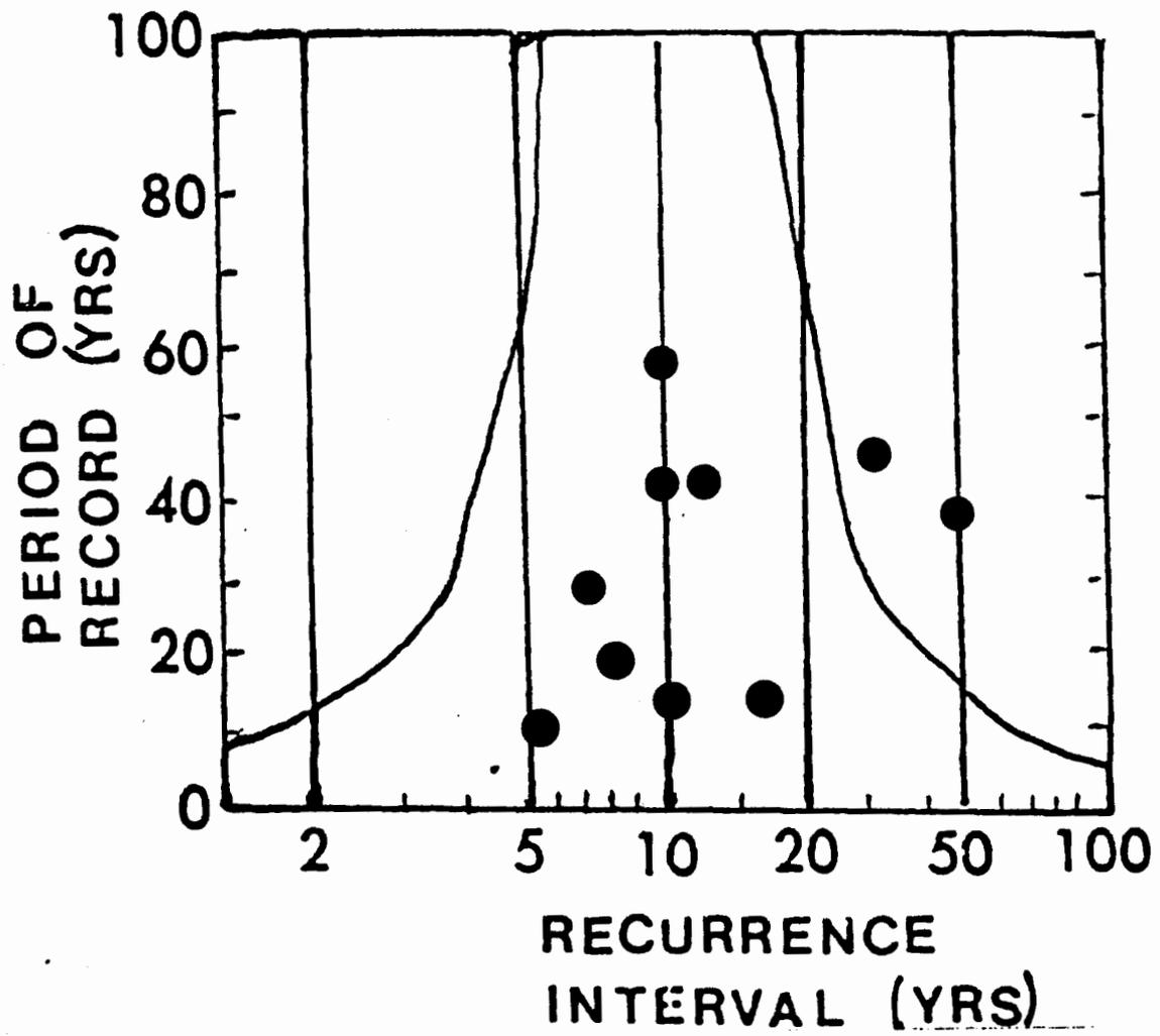
Figure 17. Homogeneity test plot for rivers in southeastern Massachusetts and northeastern Rhode Island. Data points of recurrence interval versus period of record falling within the test plot curves indicate rivers in a homogeneous hydrologic region.
