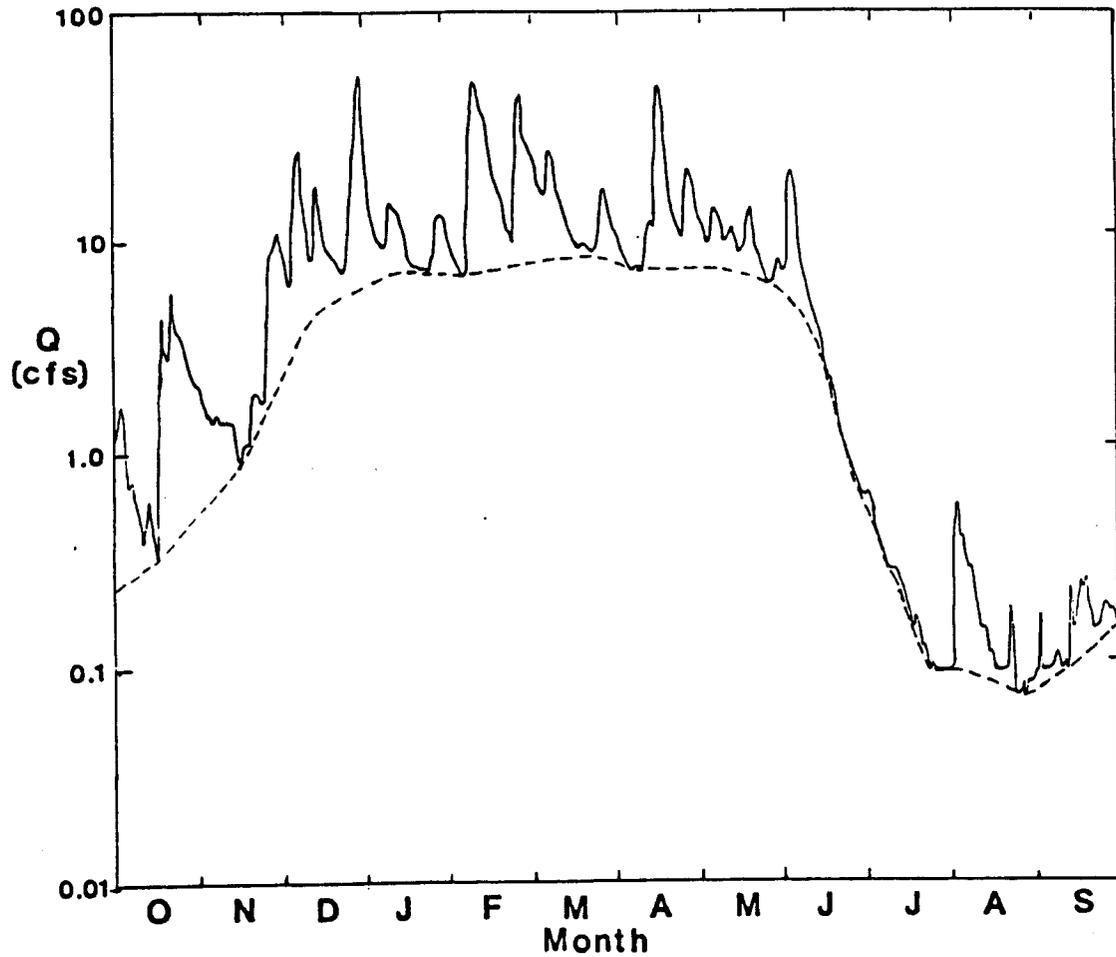
Figure 10. Annual hydrograph for Adamsville Brook, RI, for Water Year 1965, showing the yearly fluctuation in stream discharge (solid line) and in groundwater baseflow (dotted line). This Water Year was a particularly dry year.
