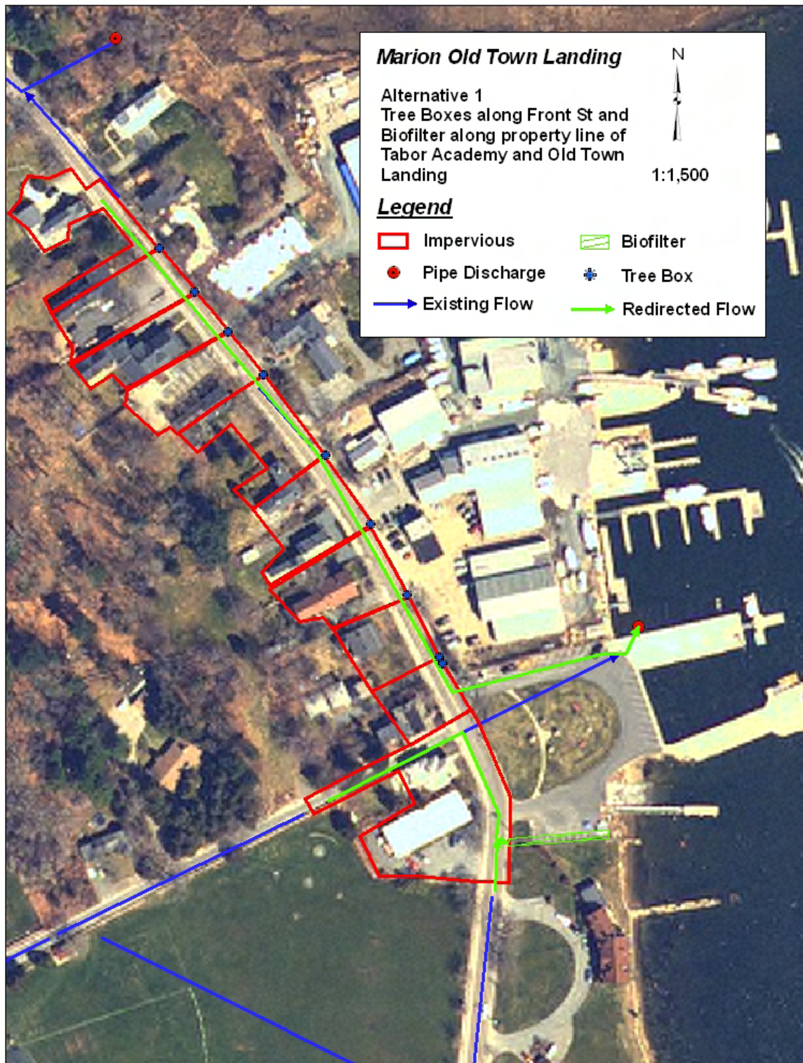
Figure 2. Conceptual Design Alternative 1. Tree Boxes and a biofilter at a parking lot will be used to treat first flush.
