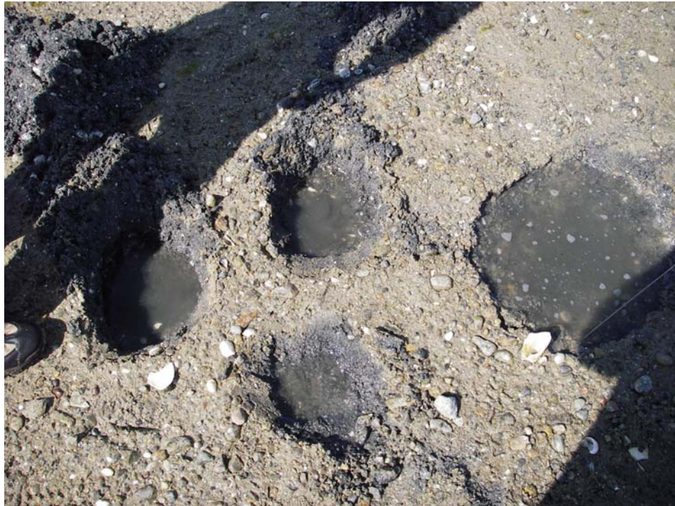
6. Test pits excavated for vertical distribution delineation.
