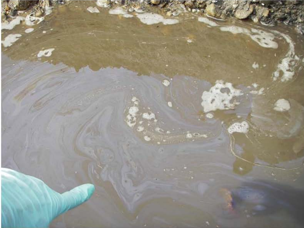
5. Sheen with flecks on water surface in trench/test pit T082508.01.
