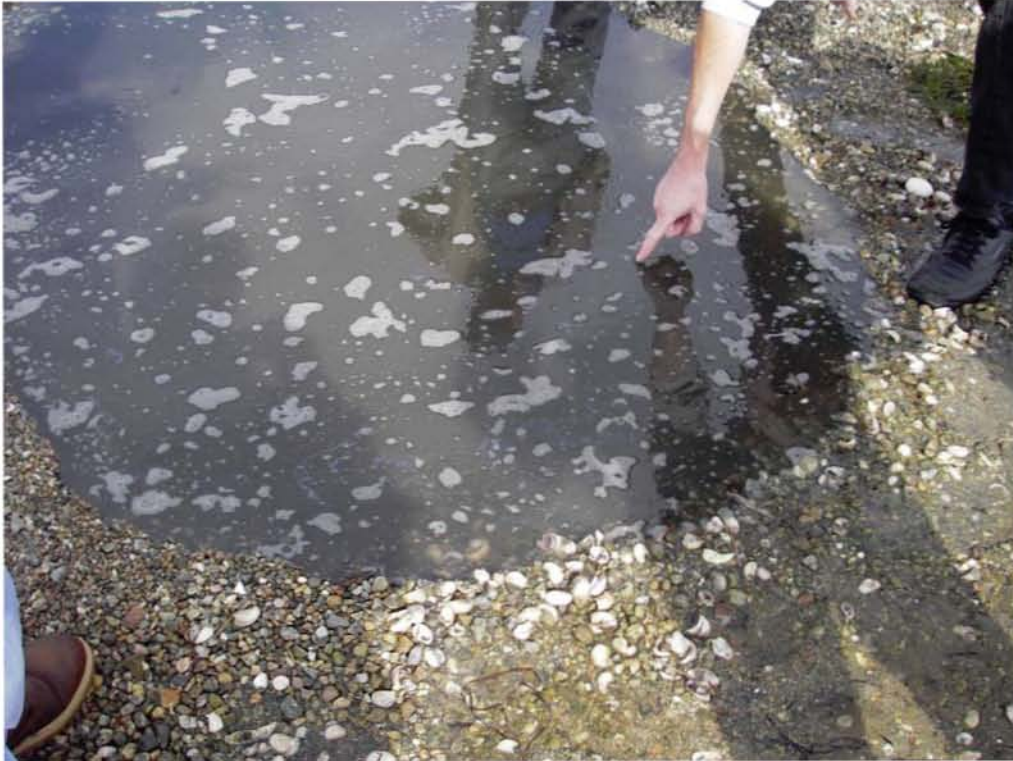
5. Test pit with faint sheen on water surface.
