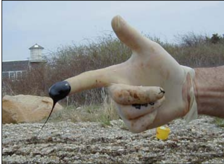
Actual clingage of cold Bouchard No. 120 oil that washed ashore 2 days after the spill. By this time, the oil had likely lost some of its most volatile constituents and was at ambient water temperature (around 44° F).
