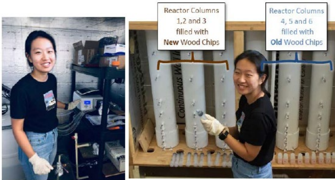
Fig. 14 PRB test Columns at the Wareham Wastewater Treatment Facility.
