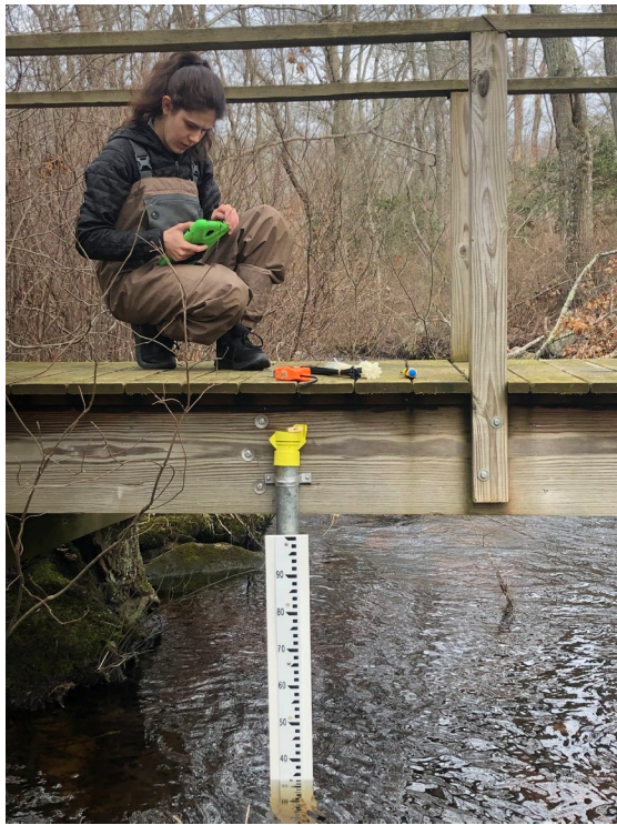
Figure 1. Image of staff gauge setup in the West Westport River on the border of Westport, MA and Little Compton, RI. Data are downloaded with a Bluetooth connection to a tablet.
