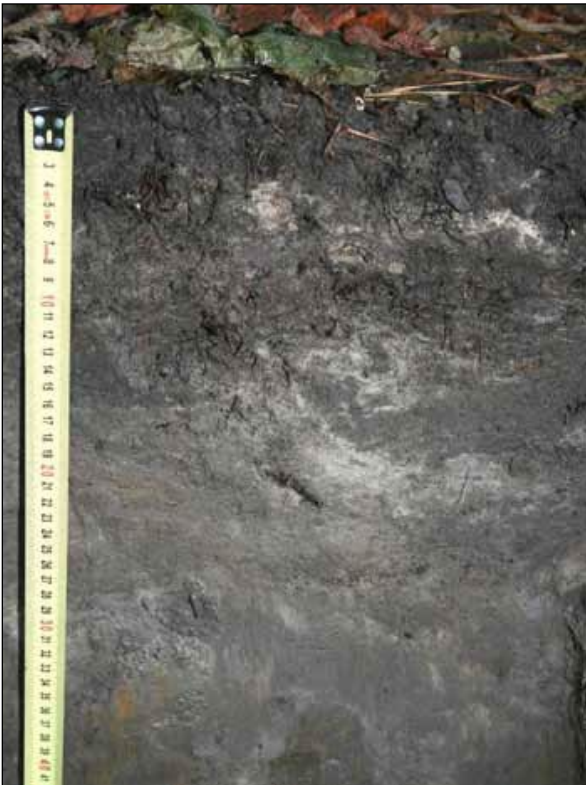
Redox depletions (lighter colored areas) are scattered within the darker matrix. Scale is in centimeters.
