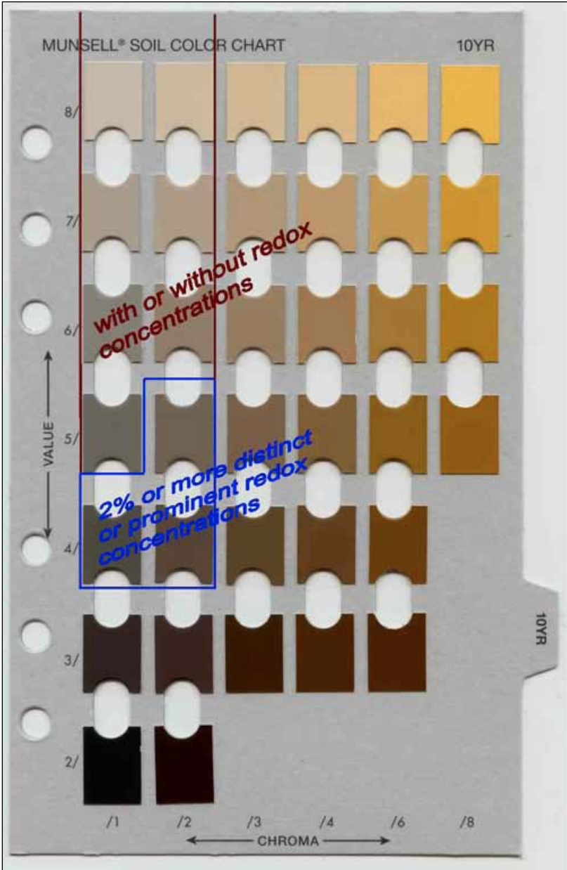
Illustration of values and chromas that require 2 percent or more distinct or prominent redox concentrations and those that do not, for hue 10YR, to meet the definition of a ACOE depleted matrix. Due to inaccurate color reproduction, do not use this page to determine soil colors in the field. Background image from the Munsell Soil Color Charts reprinted courtesy of Munsell Color Services Lab, a part of X-Rite, Inc. (Gretag/Macbeth 2000).
