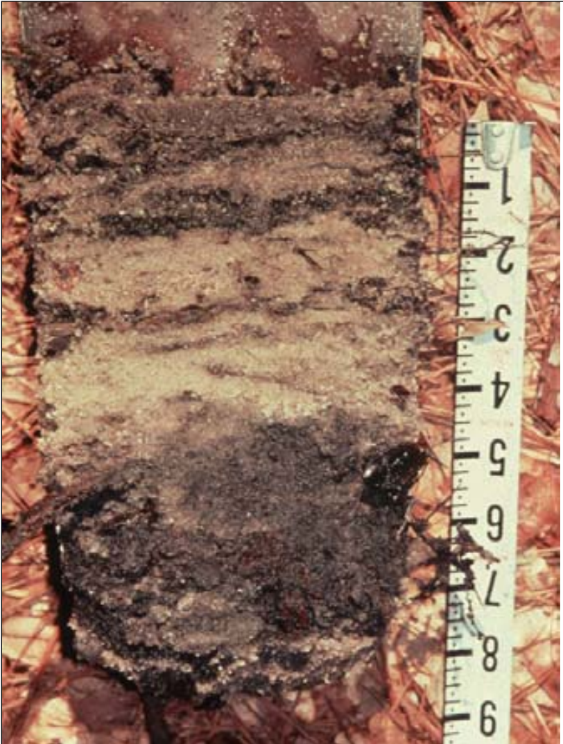
Stratified layers in loamy material. (Photo from Field Indicators of Hydric Soils )
