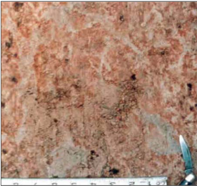
Iron-manganese masses (black spots) in a 40 percent depleted matrix. Scale is in inches.
