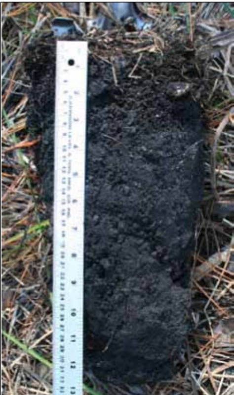
Example of Indicator S7 (Dark Surface) in a sandy soil. Scale in inches on right.
