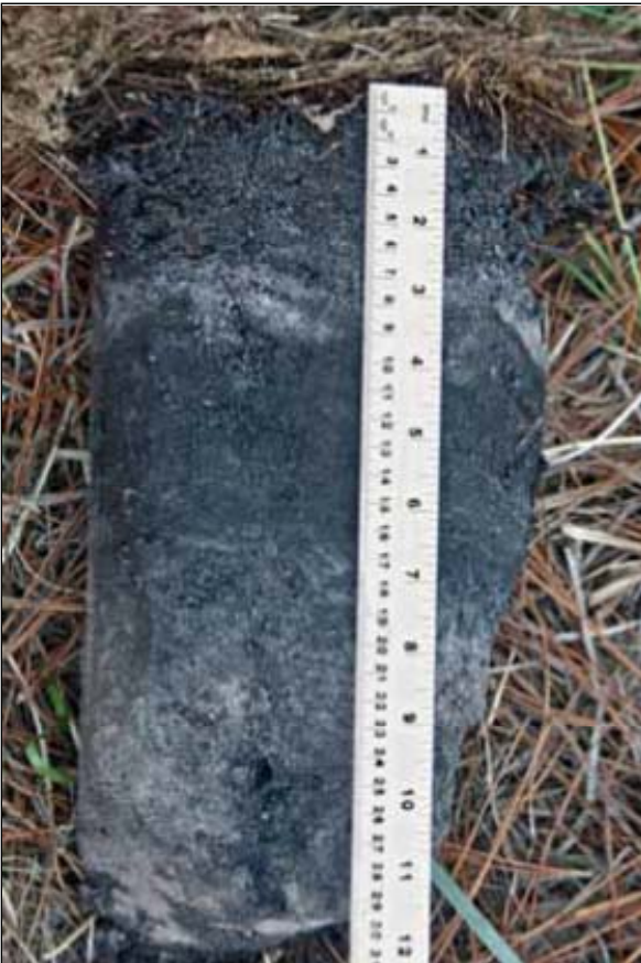
Example of Indicator S9 (Thin Dark Surface). Scale in inches on right.
