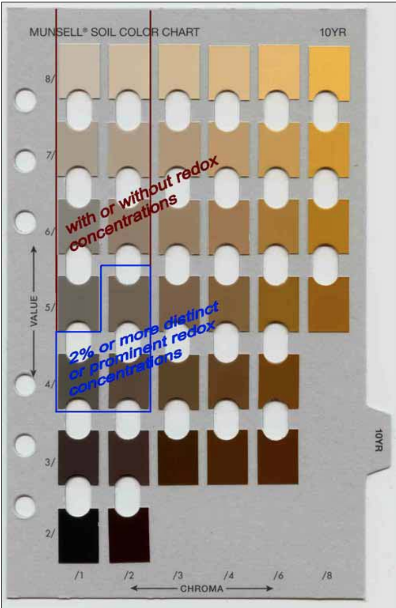
Illustration of values and chromas that require 2 percent or more distinct or prominent redox concentrations and those that do not, for hue 10YR, to meet the definition of a depleted matrix. Due to inaccurate color reproduction, do not use this page to determine soil colors in the field. Background image from the Munsell Soil Color Charts reprinted courtesy of Munsell Color Services Lab, a part of X-Rite, Inc. (Gretag/Macbeth 2000).
