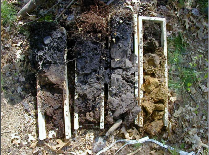
Photo credit: John Rockwell, Soil samples from Carver. Wettest from right to left. These are disturbed, sandy spodosols (evergreen forest soils). Notice the redoximorphic features in all samples.
