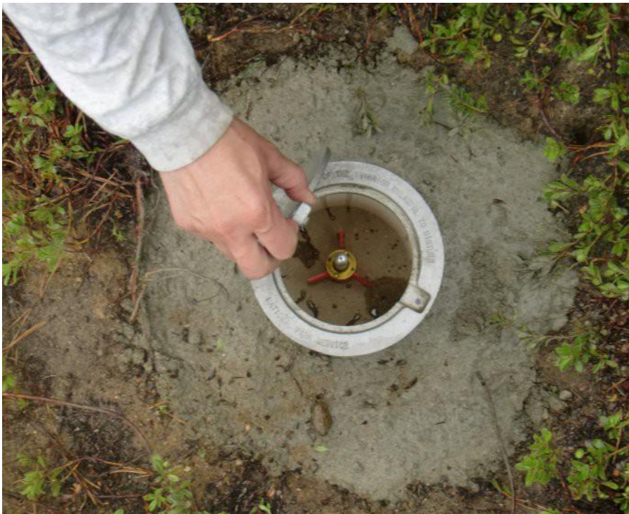
Fig. 19. A steel rod monument driven to depth with a security sleeve.
