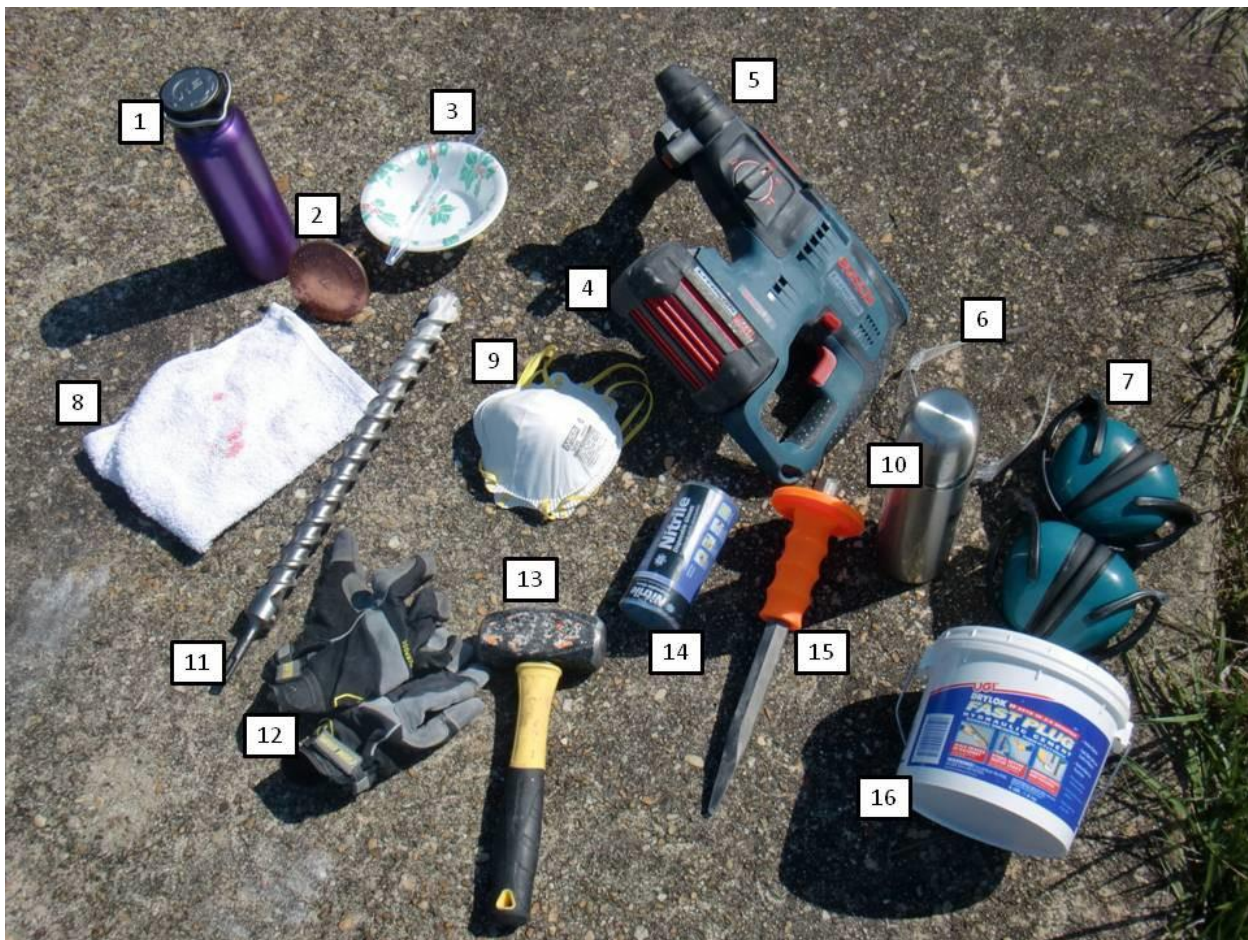
Fig. 21. Figure 4. Basic materials necessary for a brass disk drilled into bedrock or concrete. This is not a comprehensive list. Please see text for details and model numbers (where appropriate). 1. Water bottle; 2. Brass disk; 3. Disposable quart container for mixing cement; 4. Cordless battery for drill; 5. Hammer drill; 6. Eye protection; 7. Ear protection; 8. Rag; 9. Disposable face mask; 10. Water bottle; 11. Drill bit; 12. Work gloves; 13. Sledge hammer; 14. Disposable latex gloves; 15. Rock chisel; 16. Hydraulic cement.
