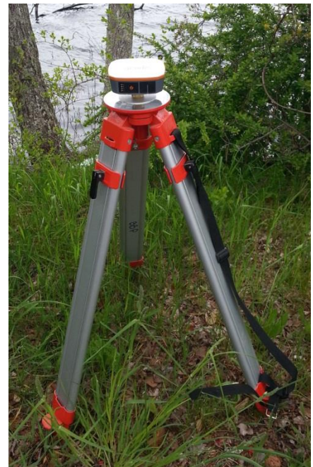
Fig. 13. One Juniper Systems Geode™ unit installed on a tripod over the benchmark, and another rover GPS on a monopod (not shown), to allow for differential GPS calculations.
