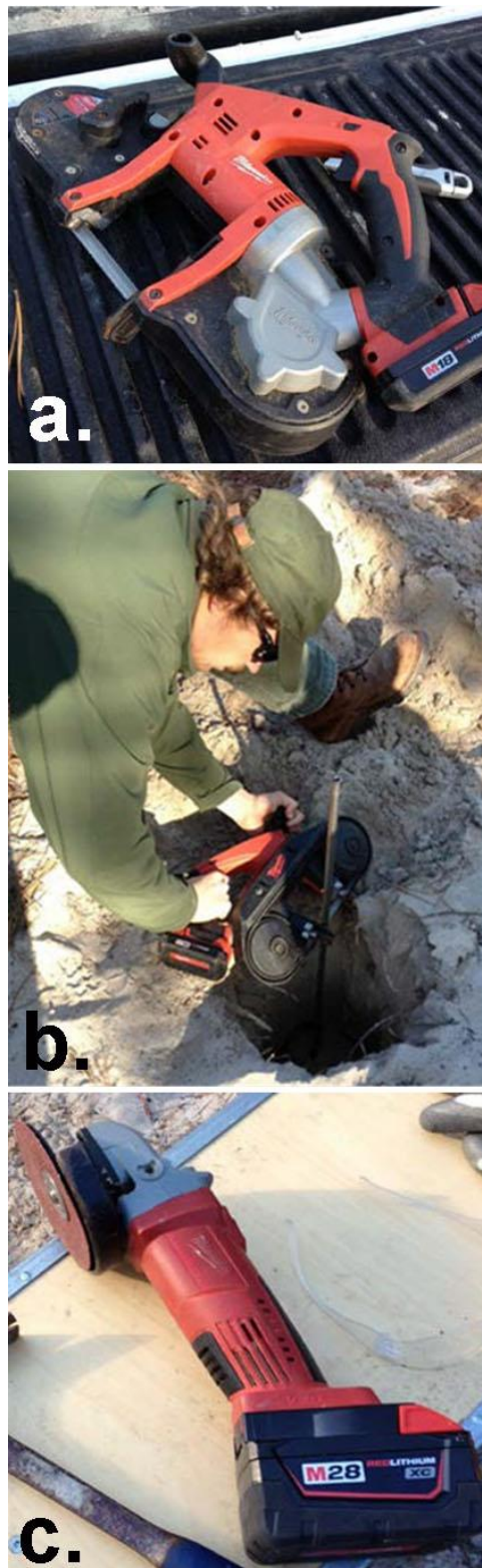
Fig. 31. If necessary, a portable band saw (a) can be used to cut the rod (b) if it has been driven to refusal. A portable power grinder (c) can then be used to round the datum point.
