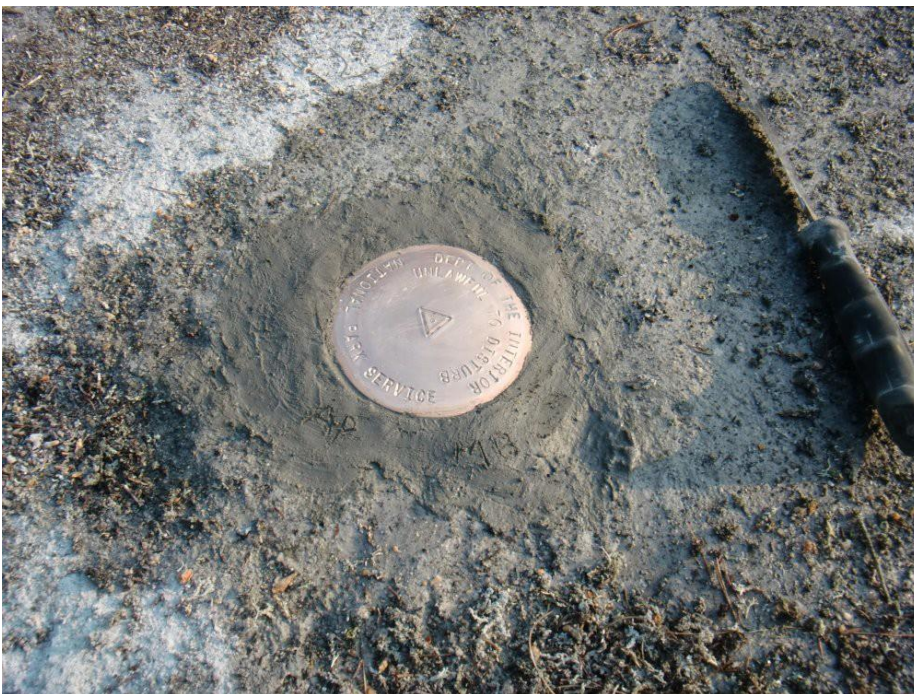
Fig. 20. Figure 3. A brass disk drilled into bedrock.
