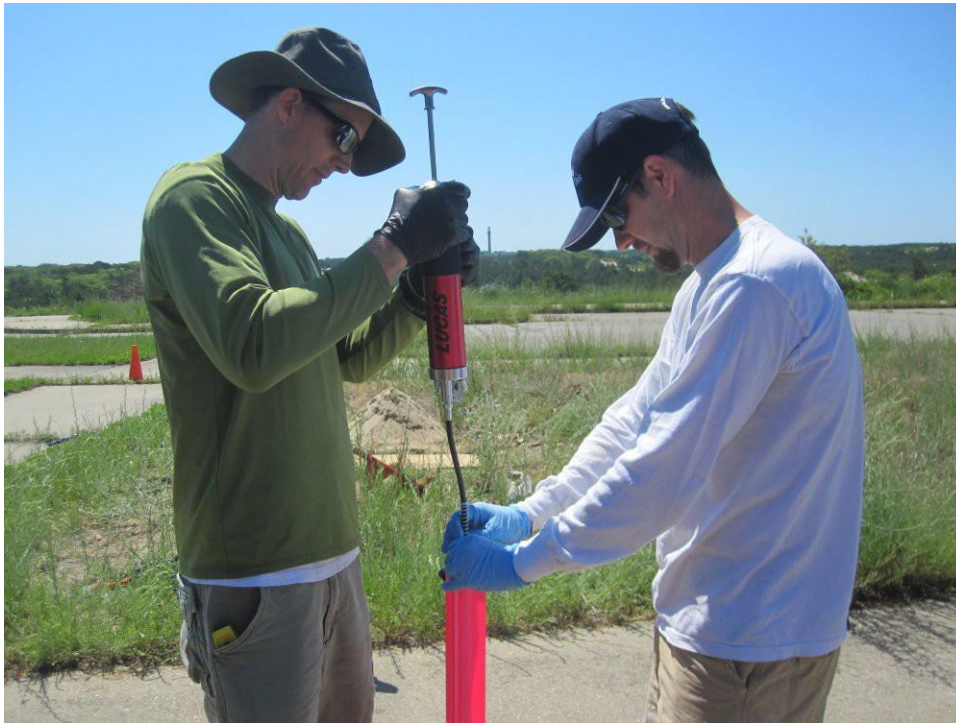
Fig. 27. Figure 10. Use a grease gun to fill the security sleeve.
