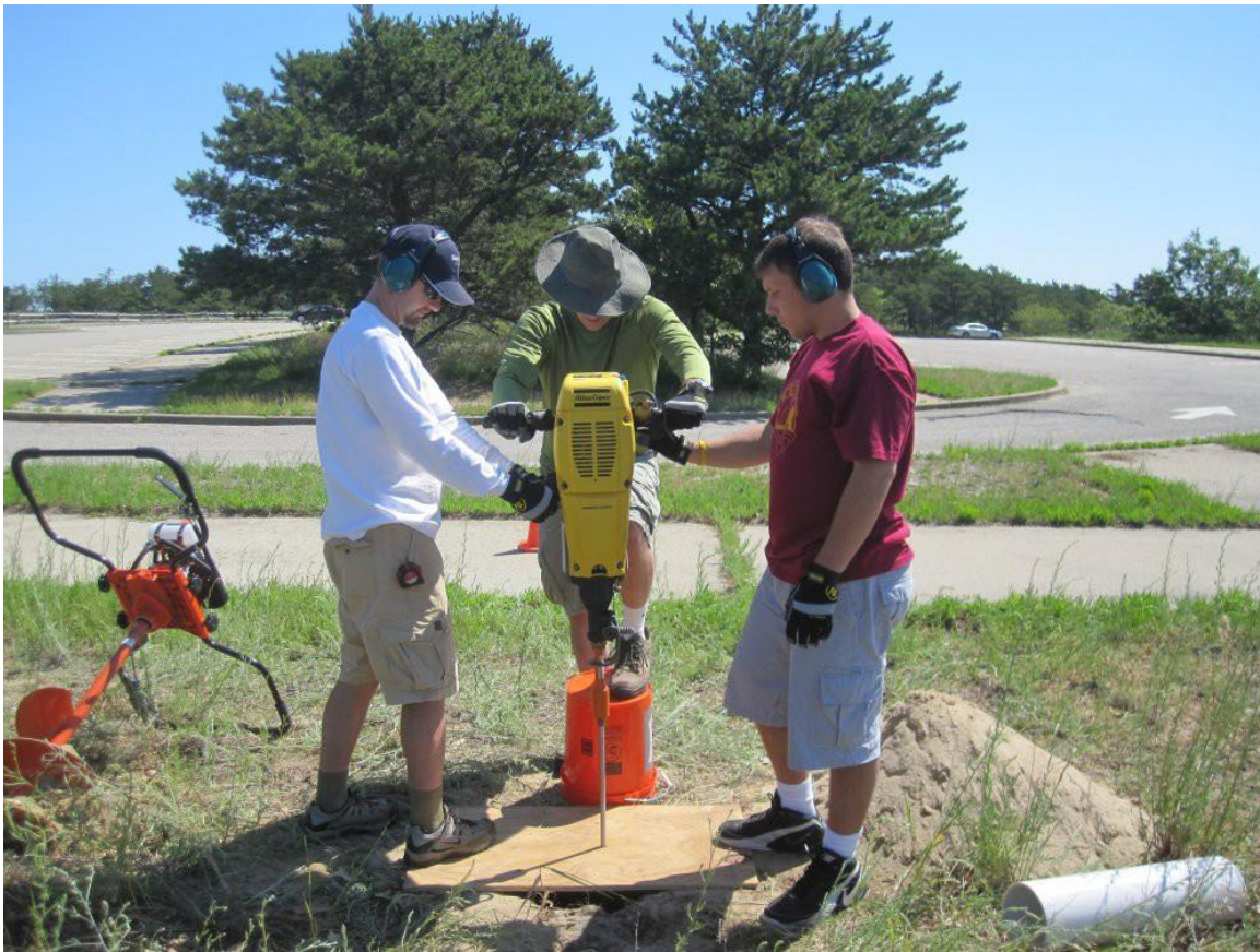
Fig. 29. Using a gas powered jackhammer, drive the rods into the ground (video).
