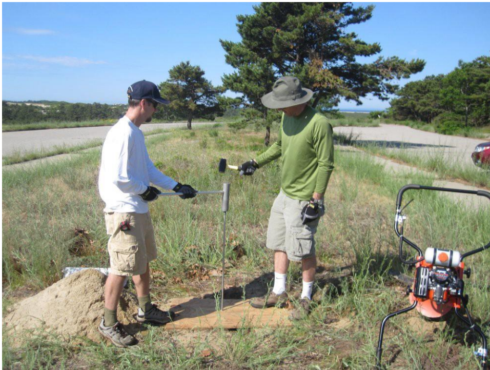
Fig. 28. Figure 11. The plywood helps stabilize the rod in the hole during manual and power driving.
