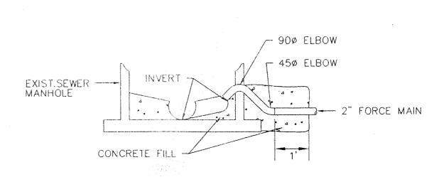
FORCE MAIN CONNECTION WITH GRAVITY SEWER
