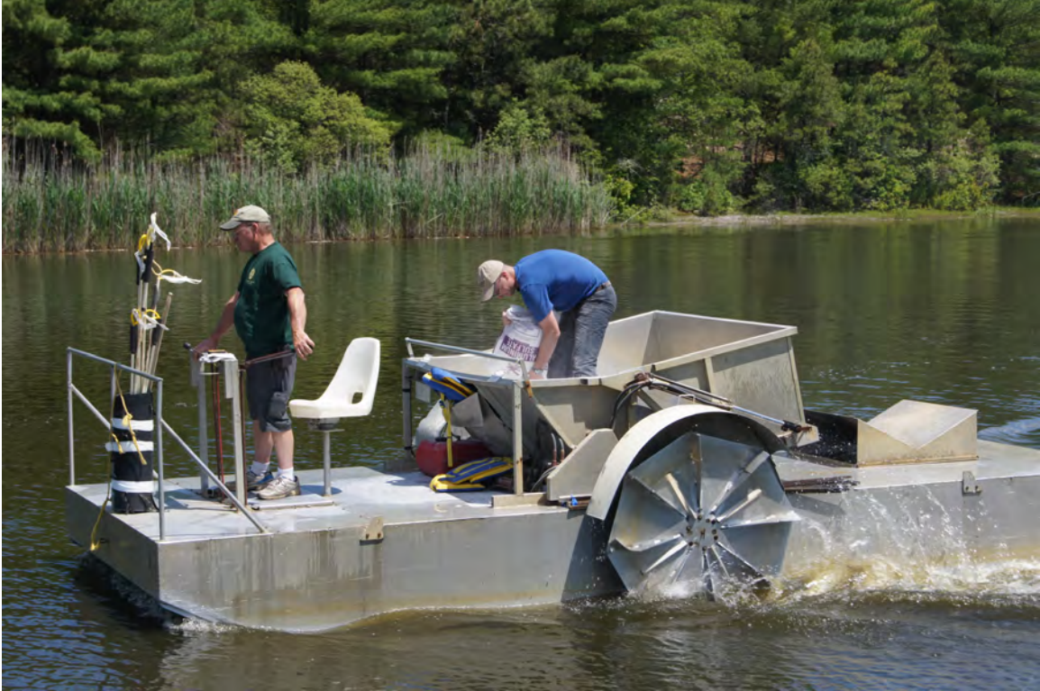
Fig. 7. Sand barge used in the application of alum to Edwards Pond West on June 15, 2016.
