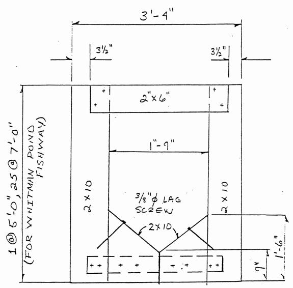
NOTE: WOOD BAFFLES SHALL BE NO.2 SOUTHERN PINE AND SHALL BE UNTREATED.
