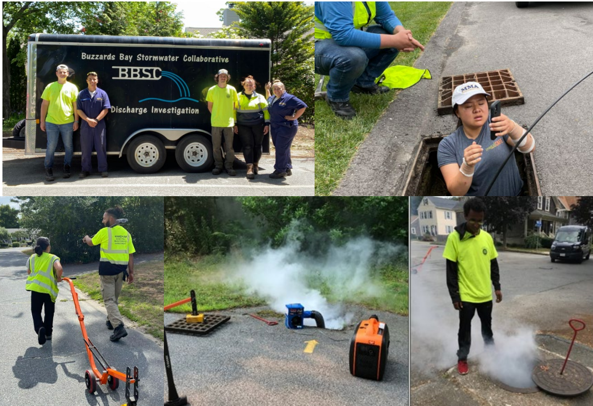
Massachusetts Maritime Academy students participating in the Buzzards Bay Stormwater Collaborative working with a municipal public works employees on an illicit discharge investigation of a municipal stormwater network.
