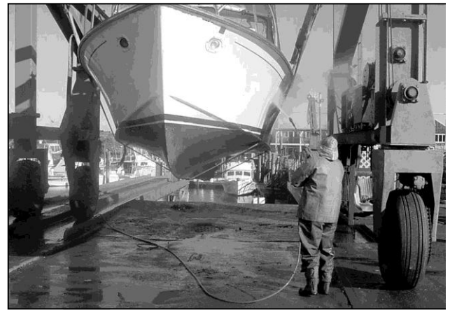
Figure 45. Pressure washing at a marina with a water collection and treatment system.
